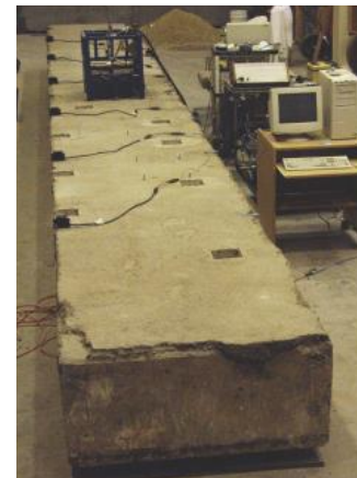
b- The dynamic test set-up for the removed prestressed concrete box girder
