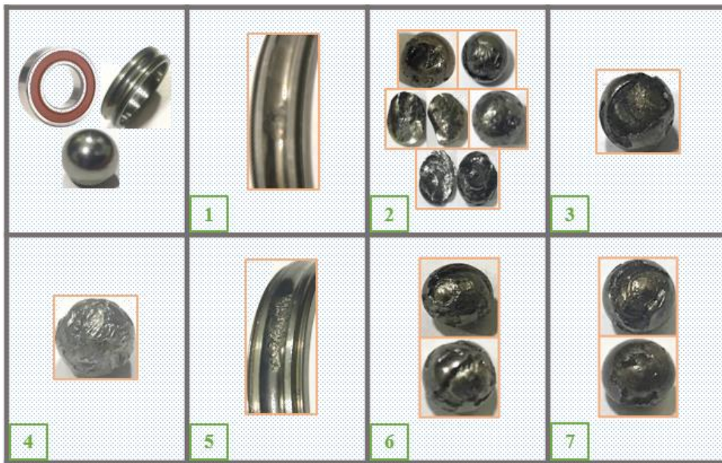
Fig. (2) Visual inspection results of failures in the elements of accelerated life test REBs
