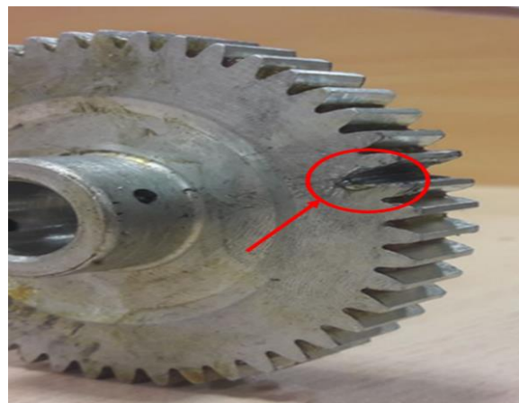
Fig. (13). Tooth crack fault
