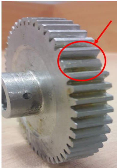
Fig. (16). Missing tooth fault
