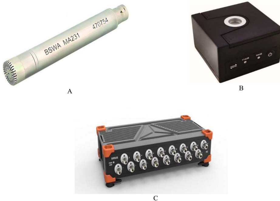
Fig. (7) A) Microphone; B) Calibrator; C) Data acquisition
