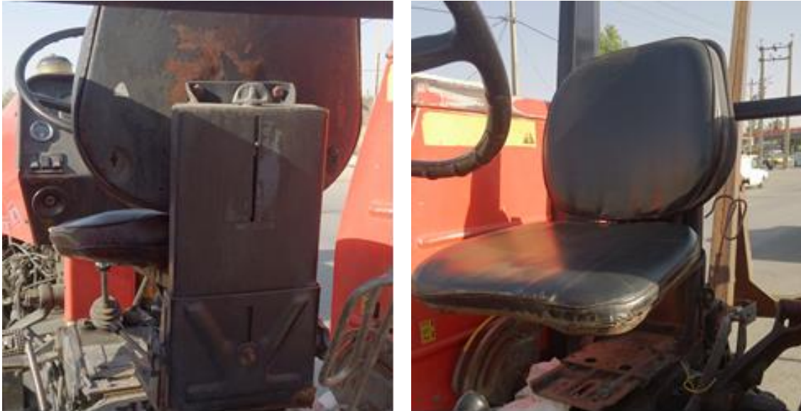
Fig. 3: Improved seat suspension (Damper Coefficient=130 N.s/m, Spring constant=8000 N/m, Mass=16
