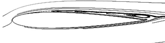
Fig. 7. (b) Streamlines on flexible airfoil at AOA of 8^\circ , Re=5000
