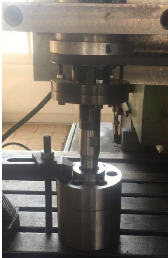
Fig 2: Test set-up used to measure the influence of ultrasonic vibration on prepared samples.
