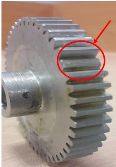
**Fig. (16).** Missing tooth fault
