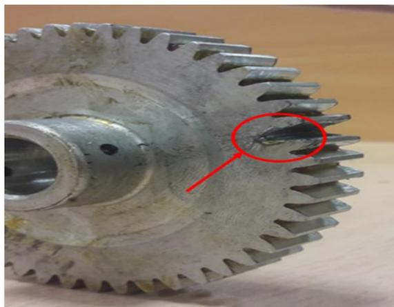
**Fig. (13).** Tooth crack fault
