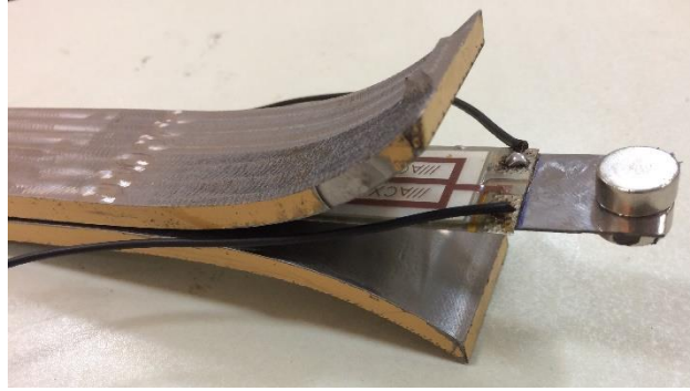
Fig. 9. Optimized nonlinear piezoelectric harvester with curved supports
