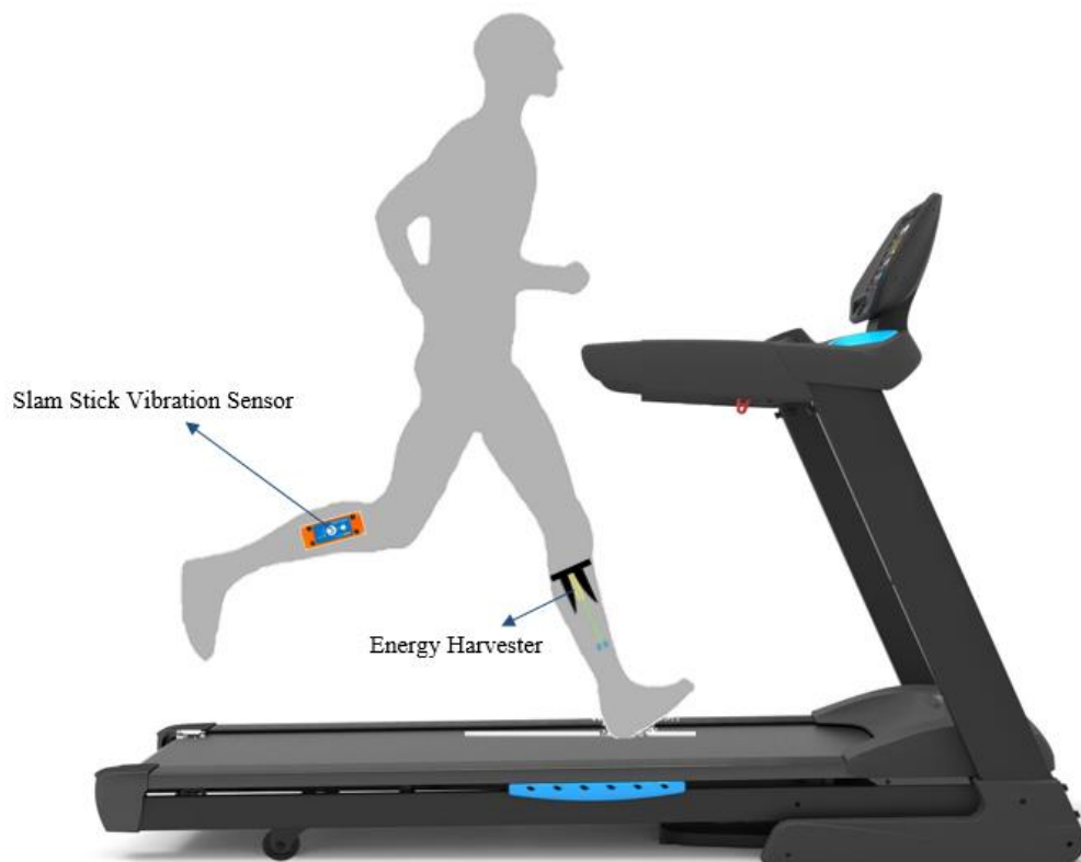
Fig.10. The schematic of the nonlinear energy harvester test setup
