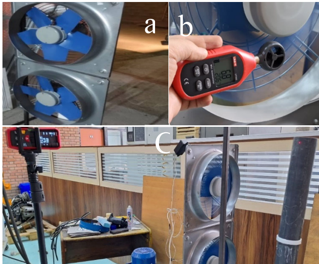
Fig. 19: Simulator fan (a), anemometer (b) Laser distance meter (c)
