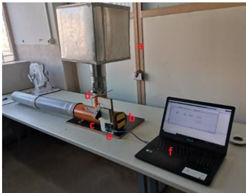
Fig. 2. The experimental setup a) Resonator b) Sound source c) Servomotor d) Butterfly and lever and f) Computer and MATLAB Software
