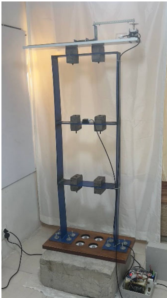
Fig. 13. Sensor placement at point M, center of the second-story beam
