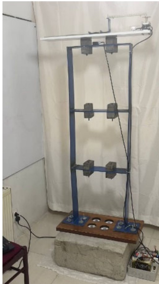
Fig. 11. Sensor placement at point J, center of the third-story beam
