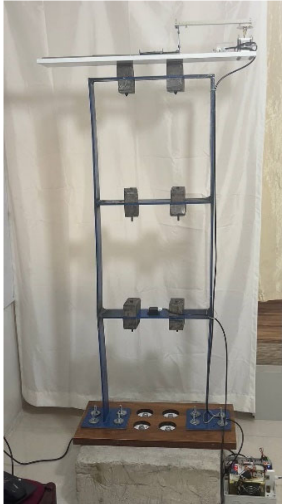
Fig. 7. Sensor placement at point P, center of the first-story beam
