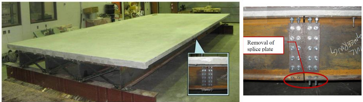
Fig2. One-third scale of composite deck and removal of the splice for damage scenario [24].
