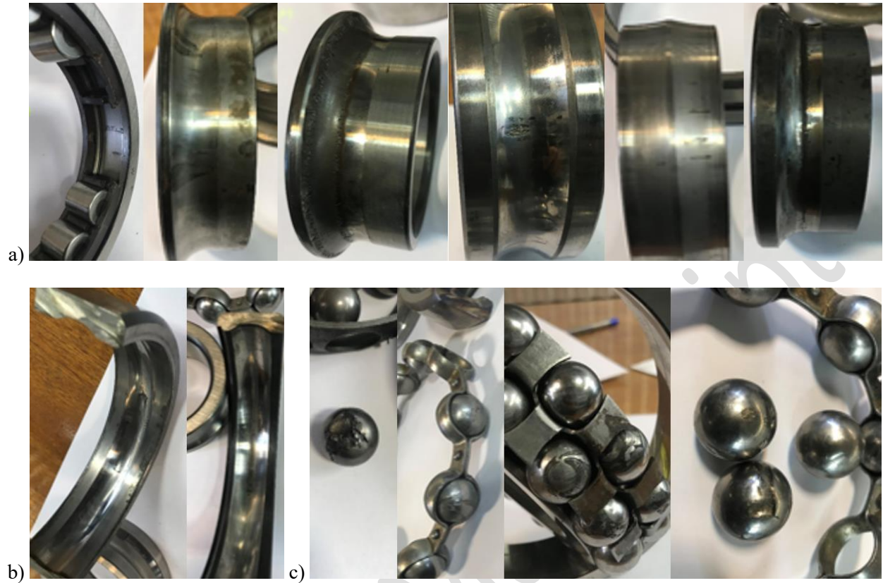
Figure 7. Visual inspection results of selected industrial REBs, showing examples of (a) Inner Race Fault (IRF), (b) Outer Race Fault (ORF), and (c) Rolling Element Fault (REF).
