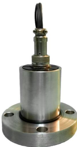
Figure 7. The final prototype of the vibrometer sensor (left); prepared test stand to conduct the experimental performance evaluation (right).
