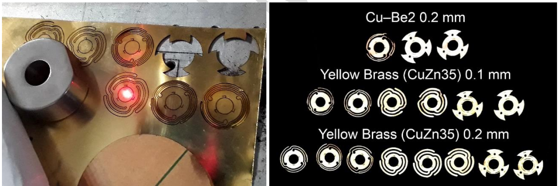
Figure 3. left) Spring production process using precision laser cutting; right) Fabricated springs with different materials and geometries
