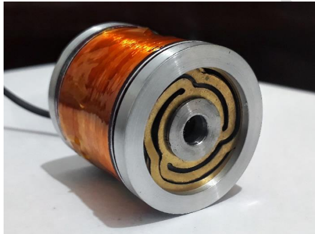
Figure 6. Assembled signal generator unit including magnet, springs, and coil
