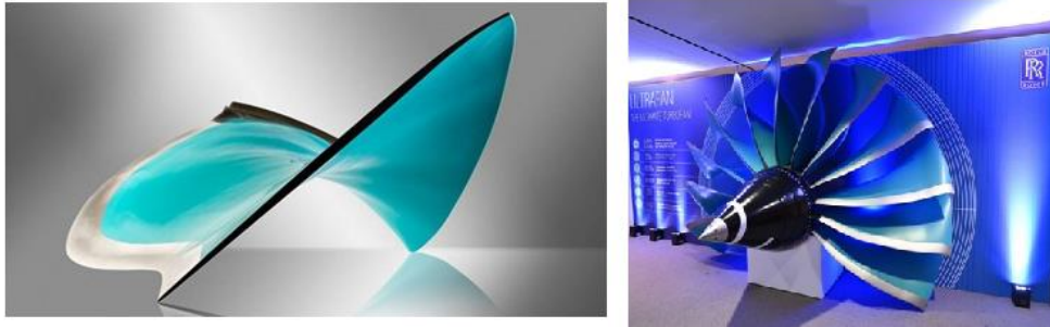
Fig. 10. Pre-twist of the Rolls-Royce UltraFan blade [47]
