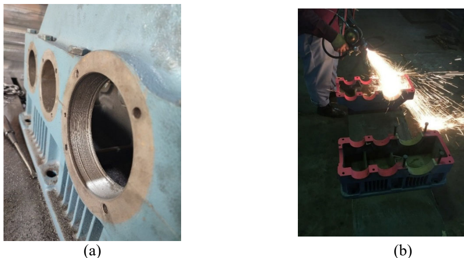
Fig.3. Metal spray welding process: a) Undercutting, b) Metal spraying, c) Welded area, d) Final area (after final machining)
