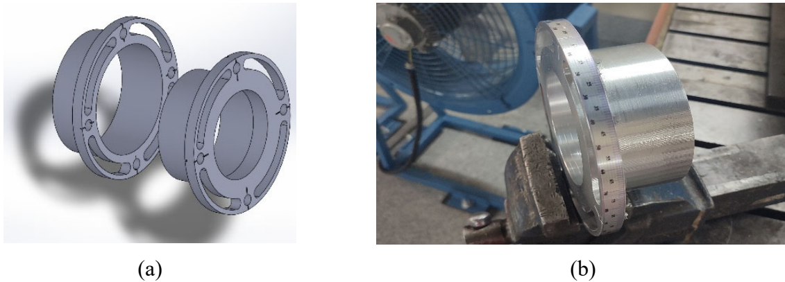
Fig.5. Eccentric end covers: a) SolidWorks model, b) constructed.
